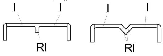
RUO: The reinforcement is connected to only one plate with type I.
