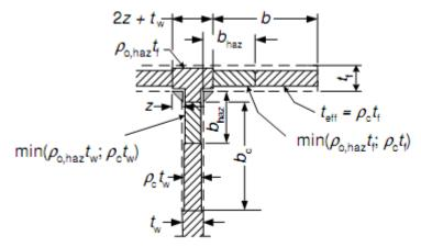
The section properties are then recalculated based on the reduced thicknesses.
