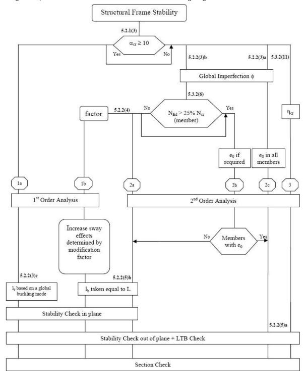
The general procedure for EC-EN1999 is shown in the following diagram.
