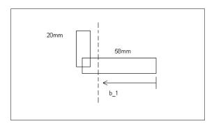
$$b_1 = \frac{(58 \times 2) \times \frac{58}{2} + (20 \times 2) \times 58}{(58 \times 2) + (20 \times 2)} = 36,44mm$$
