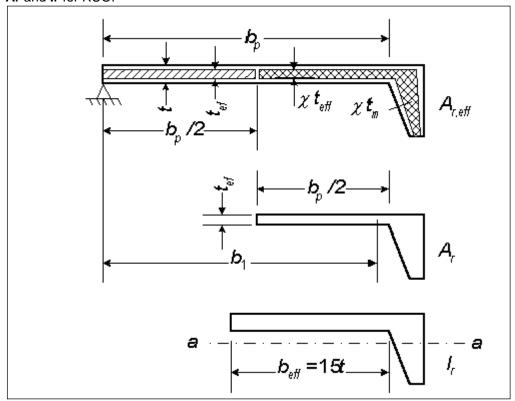
Step 3: Calculation of stiffener buckling load
