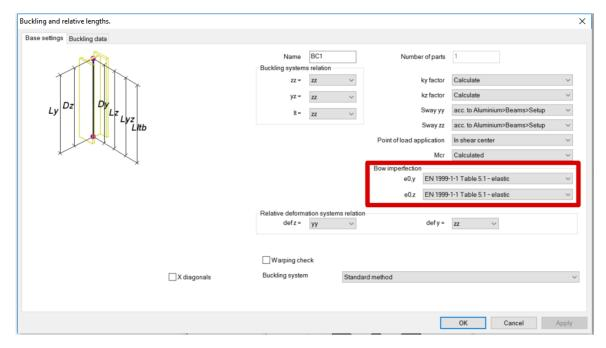
The buckling curve used for calculation of the imperfection is the curve indicated in the material properties.
