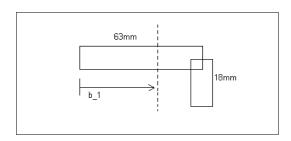
$$b_1 = \frac{(63 \times 2) \times \frac{63}{2} + (18 \times 2) \times 63}{(63 \times 2) + (18 \times 2)} = 38,5mm$$
