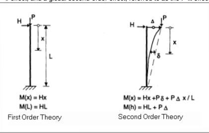
According to the EC-EN 1999, 1st Order analysis may be used for a structure, if the increase of the relevant internal forces or moments or any other change of structural behaviour caused by deformations can be neglected. This condition may be assumed to be fulfilled, if the following criterion is satisfied:
